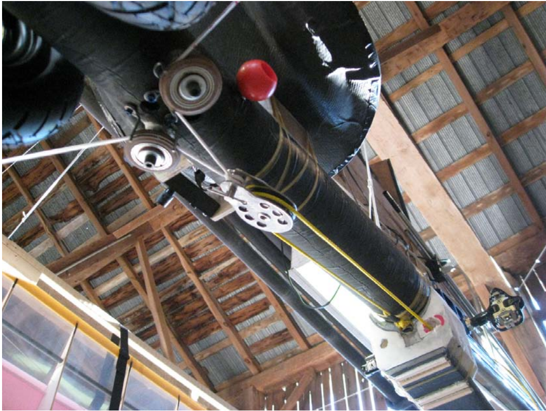
Figure 3: Drive system as seen from the bottom. The pedals attach to a Rowingbike foot-slider, which is connected to the yellow line. The yellow line goes through a 2:1 block with the two white lines turning around the pulleys and out to the attachment point on the wings.
