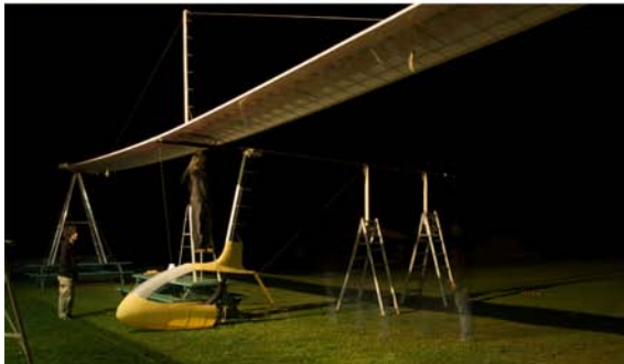
Figure 2: Photos during construction, assembly and flight testing.
