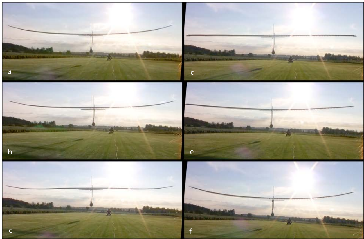
Figure 4: Wing motion during flight at various fractions of one stroke (0, 0.17, 0.41, 0.59, 0.71, 1).
